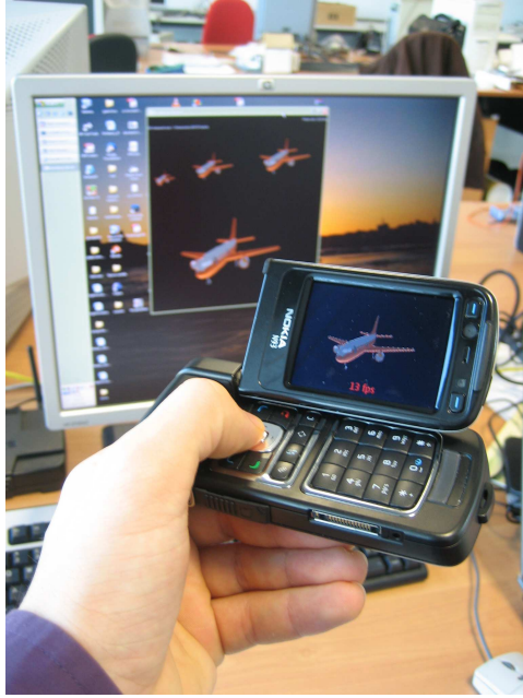
Figure 1: An example of the remote visualization session running on a Nokia N93 smartphone.
