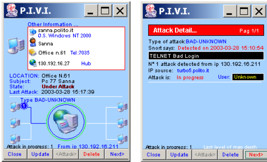
Figure 6: Details of a detected attack.
