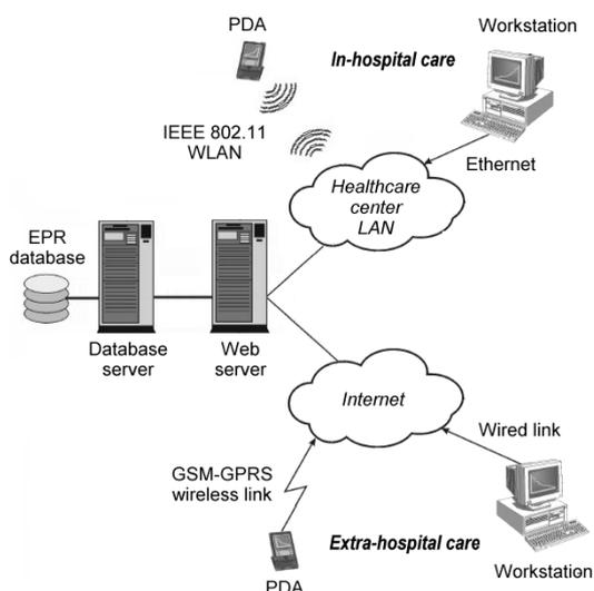
Figure 1: System overall architecture.
