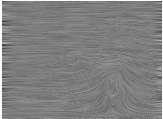
**Figure 4:** Two-dimensional laminar mixing layer visualized by LIC.
