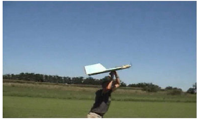
Figure 12: an example of hand launch of the UAV.
